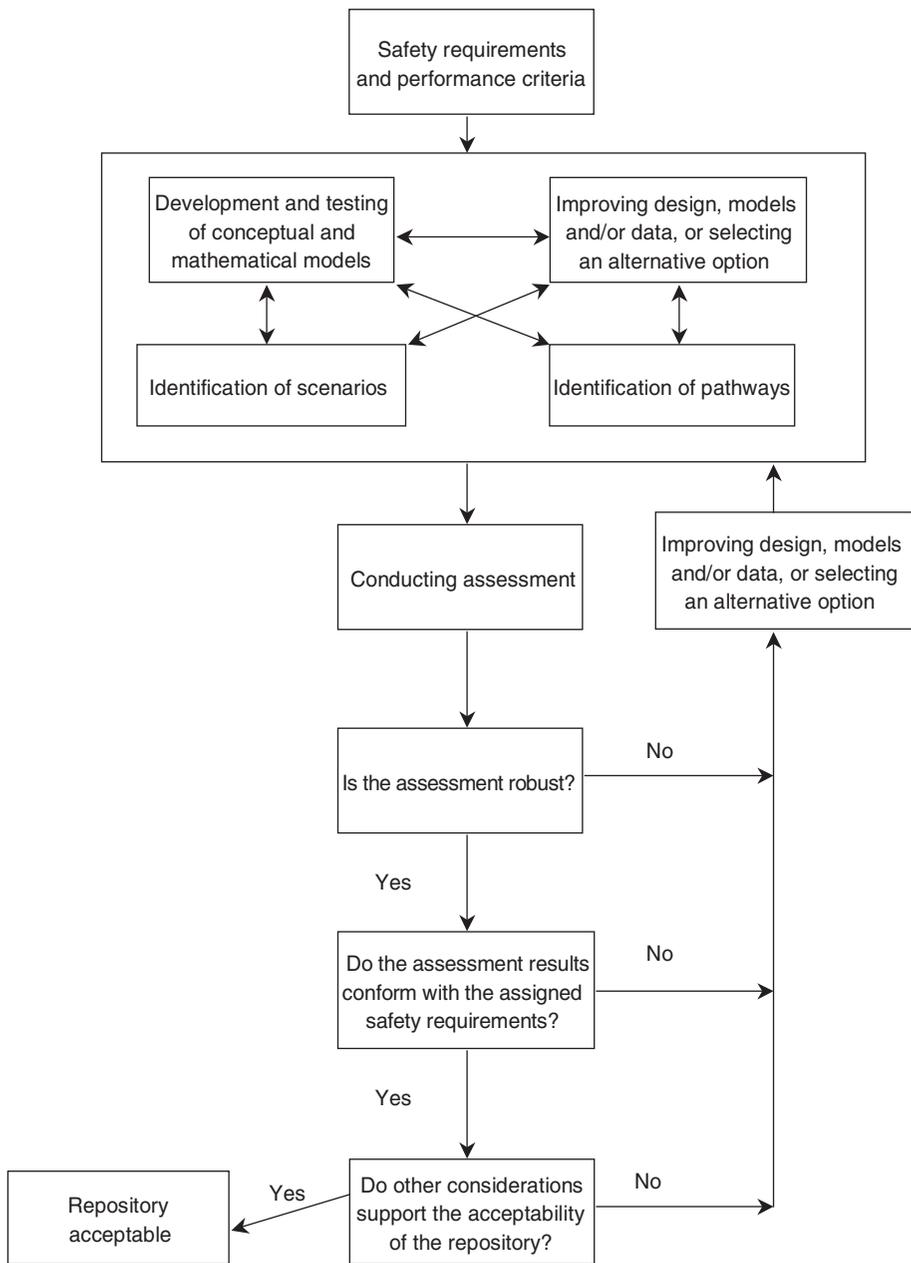
FIG. 2. Outline structure of a typical recent SA, from the system definition stage, through system analysis and interpretation, description of processes, scenario definition and analysis, to consequence analysis.
