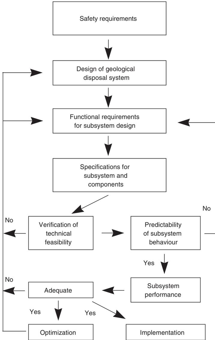
FIG. 1. Schematic illustration of the R&D programme involving SAs, PAs and engineering, as well as testing and demonstrations aimed at the implementation of geological disposal.
